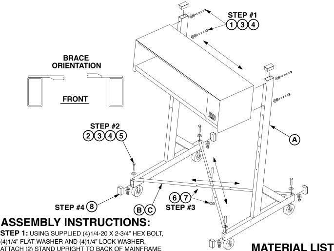
STEP 1: USING SUPPLIED (4)1/4-20 X 2-3/4" HEX BOLT. (4)1/4" FLAT WASHER AND (4)1/4" LOCK WASHER, ATTACH (2) STAND UPRIGHT TO BACK OF MAINFRAME THREADED HOLES AS SHOWN.
