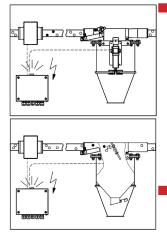
With transmitter and reciever coils an electromagnetic field is evaluated in the detector. If a metal particle enters the field the measured signal is deflected in one direction when the metal particle leaves the field the signal is defected in the opposite direction. If the detection thresholds are exceeded in both ditections a metal signal is created.
