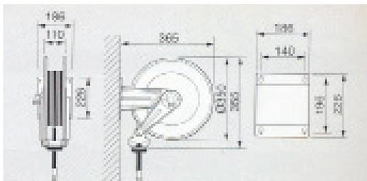
ENROULEUR CONFORME A LA NORME ATEX 94/9 -EXIIB
